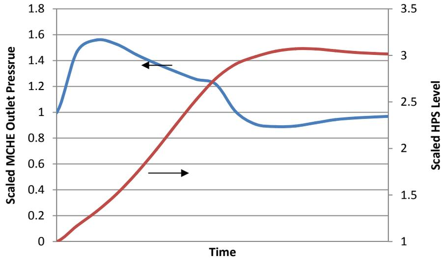
**Figure 2. Scaled MCHE Shell Pressure and HPS Level**
