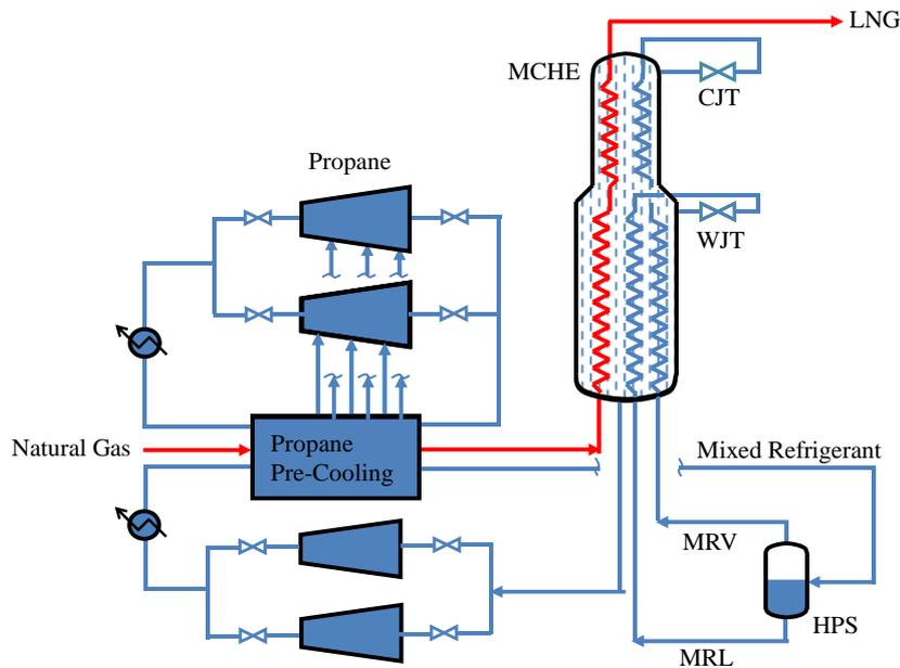
Figure 1. Simplified C3-MR Flowsheet with Parallel Compressor Strings
