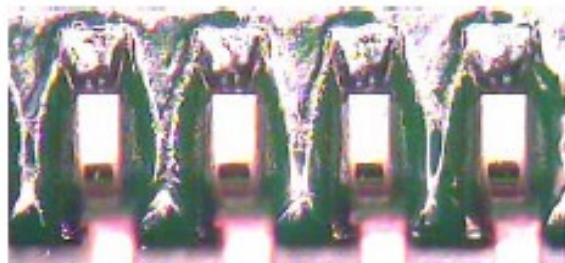
Figure 10: Pb-Sn reflow control—Sn Leads on Matte Tin Finish
