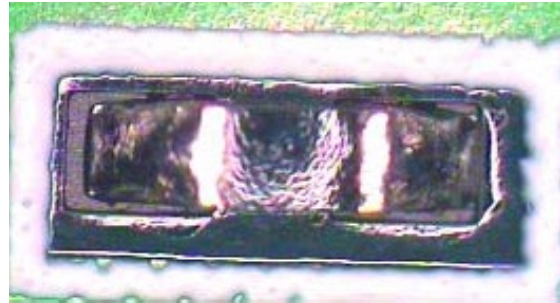
Paste A in Nitrogen—Fine Pitch Print, Ni-Pd-Au Lead—SMOBC-HASL
