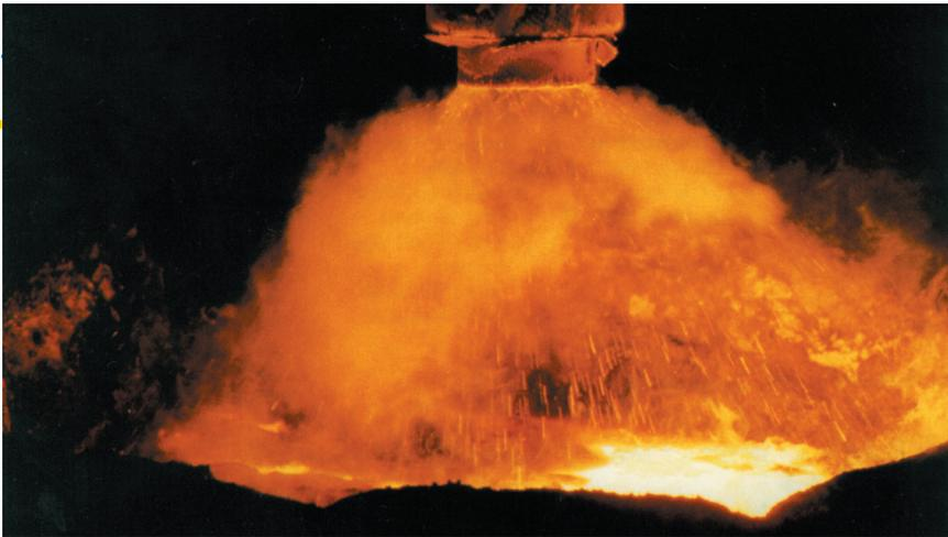
With Air Products' molten metal blanketing technologies, ferrous and non-ferrous foundries can improve casting quality, increase yields and reduce overall operating costs. These technologies, when implemented on induction and crucible furnaces, can use 50% less gas than other technologies for molten metal blanketing.
