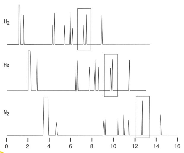
When used as a carrier gas, hydrogen typically provides higher resolution at higher linear velocities than either helium or nitrogen.
